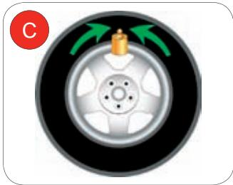
**(EN) AUTOMATIC BALANCING POSITION SEARCH:** Variable speed belt spin system to reduce operational noise and improve working lifetime and electronic shaft locking system. After the spin, the balancer automatically stops the wheel at the right weight application position.
