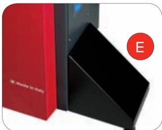
**(EN) STABILIZATION FOOT (OPTIONAL):** The standard supplied floor installation kit allows the machine to operate on wheels having maximum weight of 75 kg (165 lbs). To avoid fixing the balancer on ground, a stabilization foot KIT P is available on demand for a maximum machine wheel capacity of 50 Kg (110 lbs).
