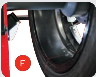
**(EN) VERSION L «LASER & LIGHT»:** Version complete with Laser line system and rim illuminator (factory installed), available for both TECO 670 and TECO 670 PLUS. If ALU programs are selected, the Laser line assists the operator during adhesive weight positioning at 6 o'clock.
